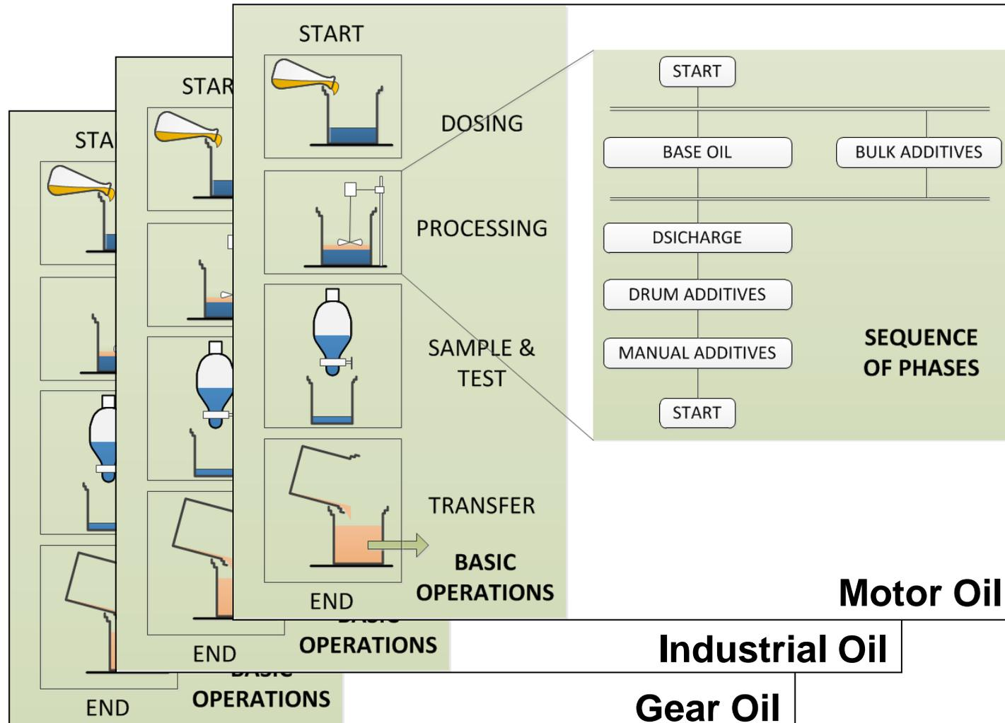
The lubricant plants are mostly designed as **‘multiple product / multiple line plants’**. High flexibility in the production can only be reached by **Automation**.
